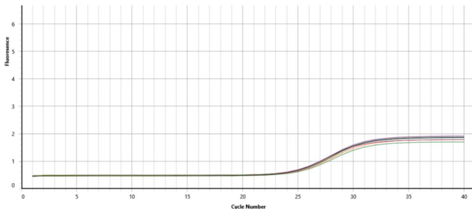
Low signals are all too often caused by old reactions left in the rotor from the previous run.
