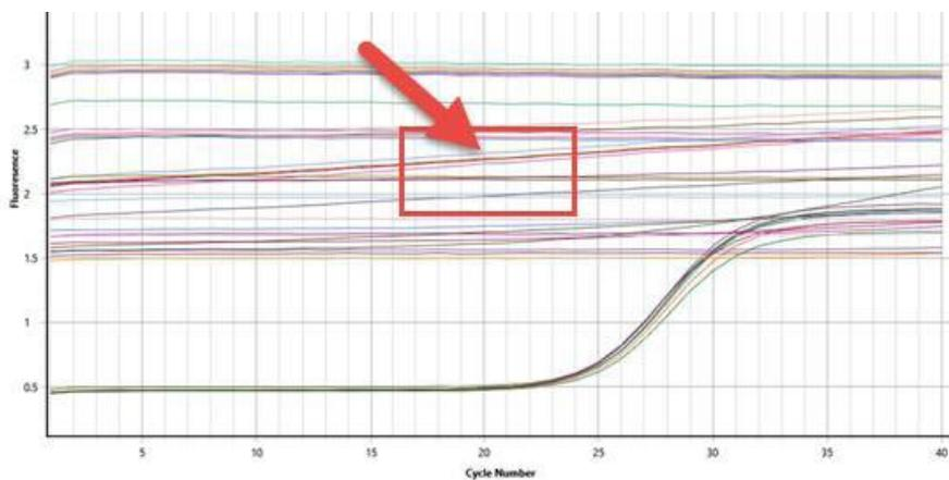
Now you can see that most of the unused reactions have a higher baseline signal. The highest signal starts at a value set for the gain adjustment (in this example it's 3 units, which is the default for intercalating dyes).
