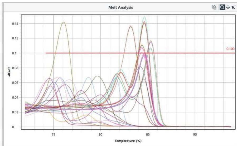
With this example, running a melt analysis, clearly shows that the higher baseline signals are indeed caused by the old reactions left in the instrument.
