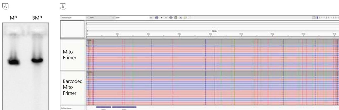
**Figure 4** A Amplification of the mitogenome with the primers containing Sequel barcodes (BMP: barcoded mito primer) does not affect the quality of the long range PCR amplicon. B SMRTbell libraries prepared with SMRTbell Barcoded Adapter Complete Prep Kit-96 (upper panel) and SMRTbell Express Template Prep Kit 2.0 (lower panel) exhibited identical variant calling.
