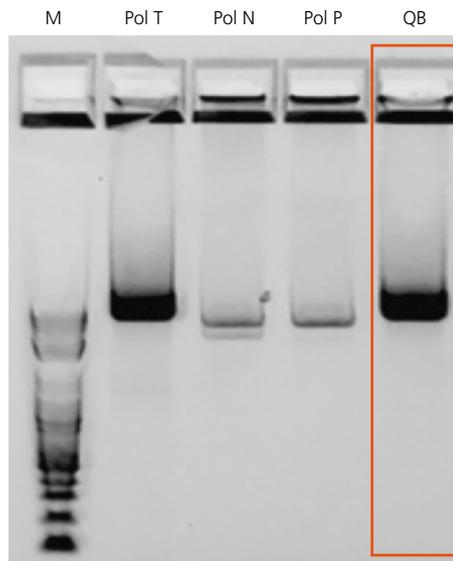
**Figure 5** Amplification of GBA gene using different polymerases.
