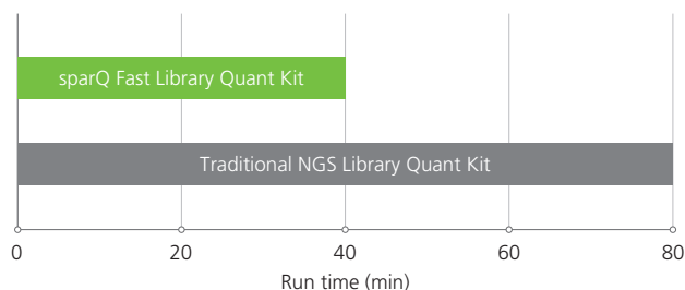
Figure 1 Comparison of average qPCR run time for library quantification. sparQ Fast Library Quant Kit uses fast cycling protocol, allowing results to be achieved in 40 minutes versus 1 hour and 20 minutes with the traditional NGS Library Quant Kit.
